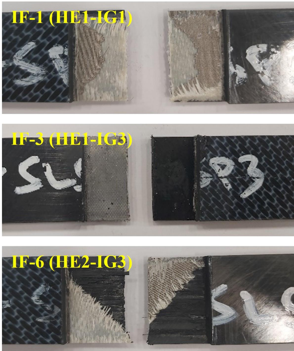
Figure 3.11 Examples of interlaminar failure modes observed during SLSS tests. From top to down: Cohesive, adhesive, mixed (cohesive and delamination).
