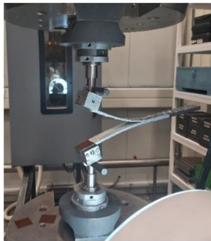
Figure 2.6 Specimen geometry (above) and Mode-I loading fixture (below) of the G_{IC} tests.
