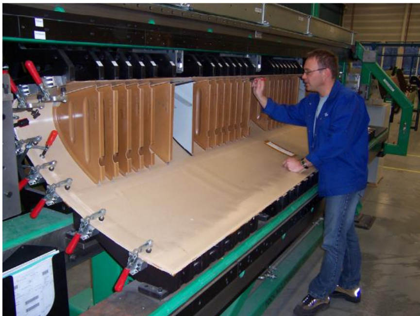
Figure 1.5 Resistance welding of ribs to the leading edge of a passenger airplane [7].
