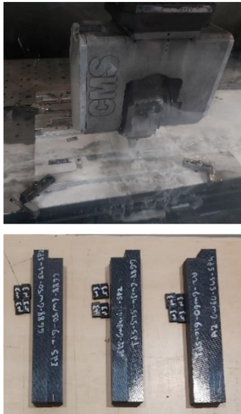
Figure 2.5 Machining operation (above) and mechanical test specimen examples after machining (below).
